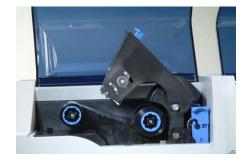
printhead bracket in a P330 $\iota$  is on a pivot system. This clever design provides better alignment of the printhead to the platen roller for enhanced print registration.
